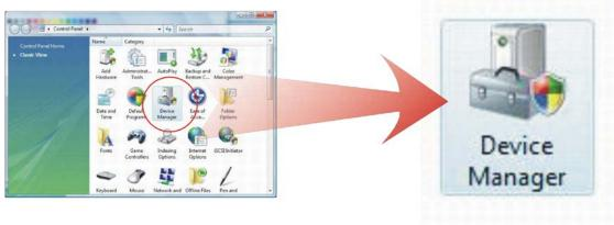
(2) In the Device Manager window, you should see this board under **Multifunction adapters** (4-port RS-232 Serial Card in this example). You should also see SUNIX COM port under **Ports** (**COM & LPT**).
