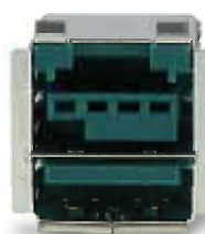
+12VDC Voltage Keyed with Teal coding
