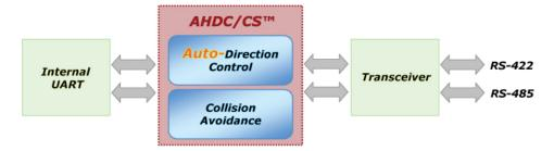
Auto Hardware Direction Control (AHDC™) technology makes it easier to manage 2-wire RS-485 half-duplex communications, eliminating the need for software interference. User does not necessary to write extra code for Windows applications to control the half-duplex protocol. Auto Hardware Direction Control (AHDC™) technology is the key feature of SUNIX UART, and this function is default enabling.
