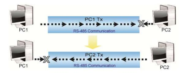
Auto Carrier Sense (ACS™) technology will check the status of RS-485 communication bus. If the bus is idle, it starts transmission. If the bus is not idle (some data flows in the bus), then it will postpone the transmission of UART until the bus is idle. Due to the reduction of TX/RX packet conflicting on RS-485 one-way traffic bus, it will enhance better system performance and RS-485 communication ability. SUNIX recommend enabling this feature.
