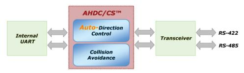
Auto Hardware Direction Control (AHDC<sup>™</sup>) technology makes it easier to manage 2-wire RS-485 half-duplex communications, eliminating the need for software interference. User does not necessary to write extra code for Windows applications to control the half-duplex protocol. Auto Hardware Direction Control (AHDC<sup>™</sup>) technology is the key feature of SUNIX UART, and this function is default enabling.
